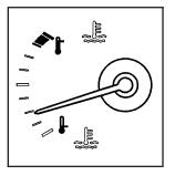
This gage shows the engine coolant temperature.
